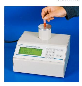
The Gamma Counter LG-1 is designed radioimmunoassay (RIA) and immunoradiometric assay (IRMA) in medium and small size laboratories employing isotope <sup>125</sup>I. The counter is an easy to operate instrument with no moving mechanical components enlarging his operation reliability.
