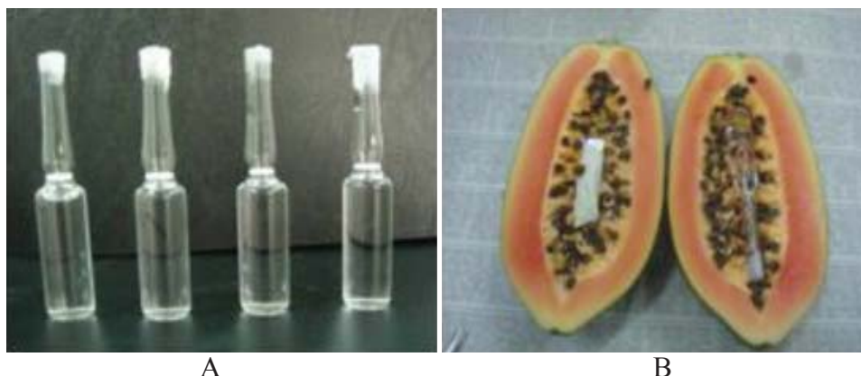
Fig.7. Fricke dosimeters: (A) as prepared Fricke solutions, (B) application of Fricke dosimeter in research related to food irradiation. (Adapted from Ref. [28]).
