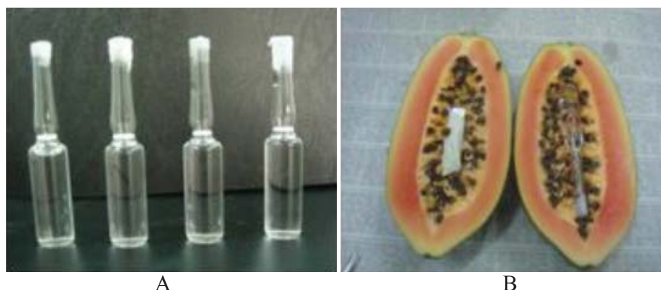
Fig.7. Fricke dosimeters: (A) as prepared Fricke solutions, (B) application of Fricke dosimeter in research related to food irradiation. (Adapted from Ref. [28]).
