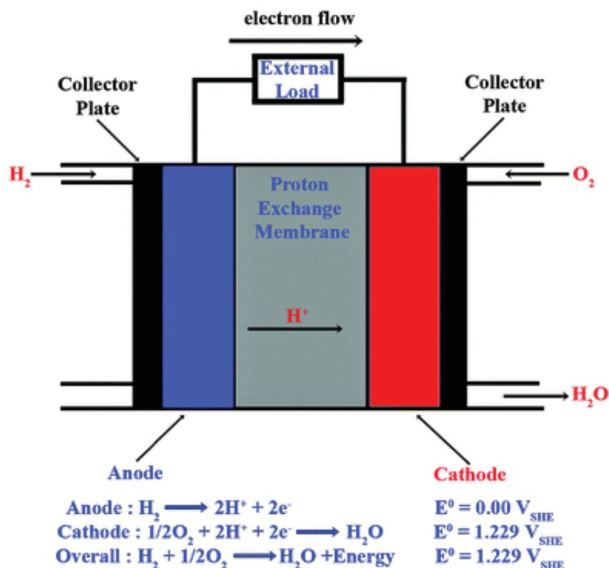
Fig.4. Sketch showing the assembly of a typical PEMFC and the electrochemical reactions involved.
