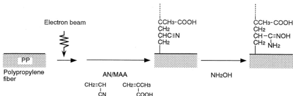
Fig. 1. A simplified scheme for the preparation of amidoxime fibers by radiation-induced grafting.
