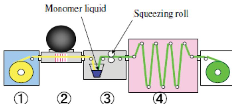
Fig.3. Schematic presentation of continuous radiation grafting system used by the Ebara Company [14] for the production of specialty membranes: 1 – trunk polymer feeding, 2 – electron accelerator, 3 – monomer impregnating zone, 4 – grafting reaction zone.
