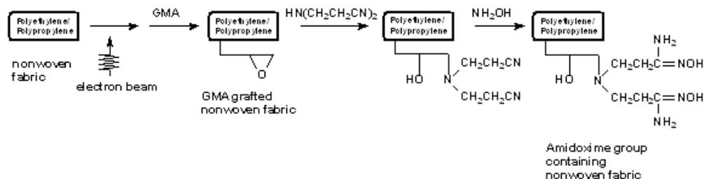
Fig.2. Scheme showing the synthesis of a novel non-woven adsorbent with enriched amidoxime groups.
