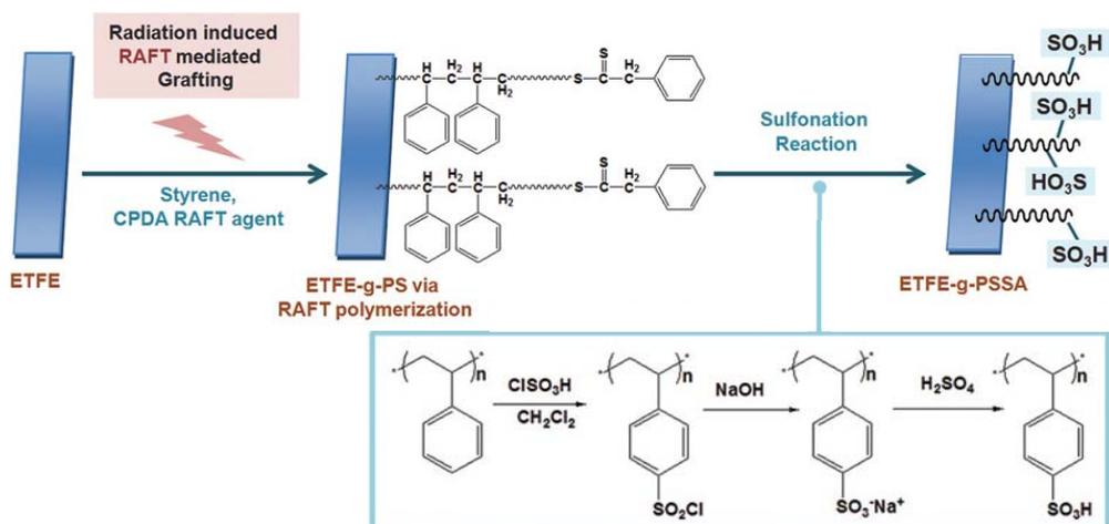
Fig.5. A scheme of the RAFT-mediated grafting process of styrene from ETFE surface and eventual sulfonation.
