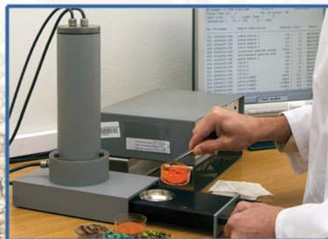
Aparat SURRC PPSL-Irradiated Food Screening System
