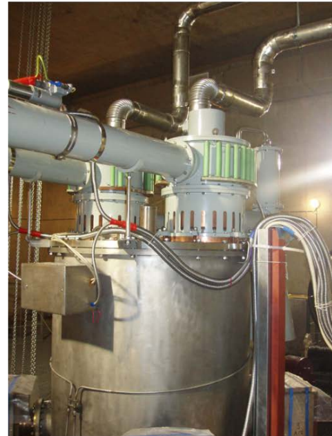
Fig. 17. RF electron accelerator type ILU-10: 1 – vacuum envelope, 2 – resonator, 3 – focusing coil, 4 – ion pump, 5 – electron gun, 6 – scanner, 7 – coupling loop support, 8 – vacuum capacitor, 9 – RF generators
