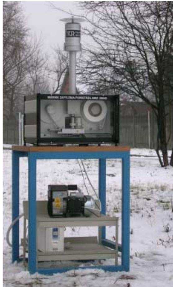
Fig.1. Airborne dust concentration gauge AMIZ-2004G.
