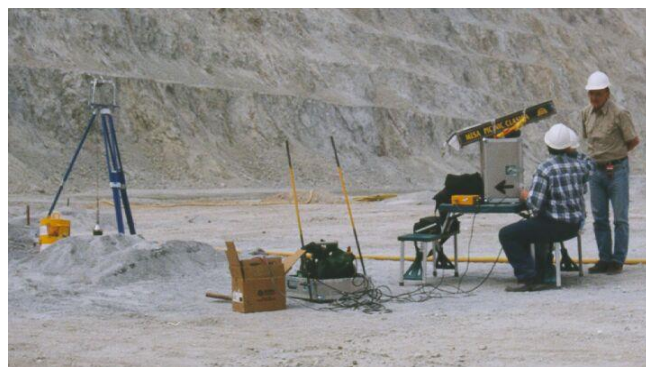
PGNAA method used for borehole logging in copper mining
