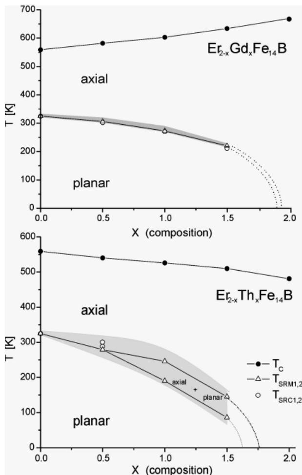
**Fig. 2.** Spin structure phase diagrams for the  $\text{Er}_{2-x}\text{Gd}_x\text{Fe}_{14}\text{B}$  and  $\text{Er}_{2-x}\text{Th}_x\text{Fe}_{14}\text{B}$  compounds.  $T_C$  – Curie temperature,  $T_{\text{SRM},1,2}$ ,  $T_{\text{SRC}}$  – spin reorientation temperatures determined from Mössbauer and DSC, respectively. The shaded area marks the coexistence of axial and planar arrangements. Dotted lines mark the probable area of coexistence of planar and axial spin arrangements.
