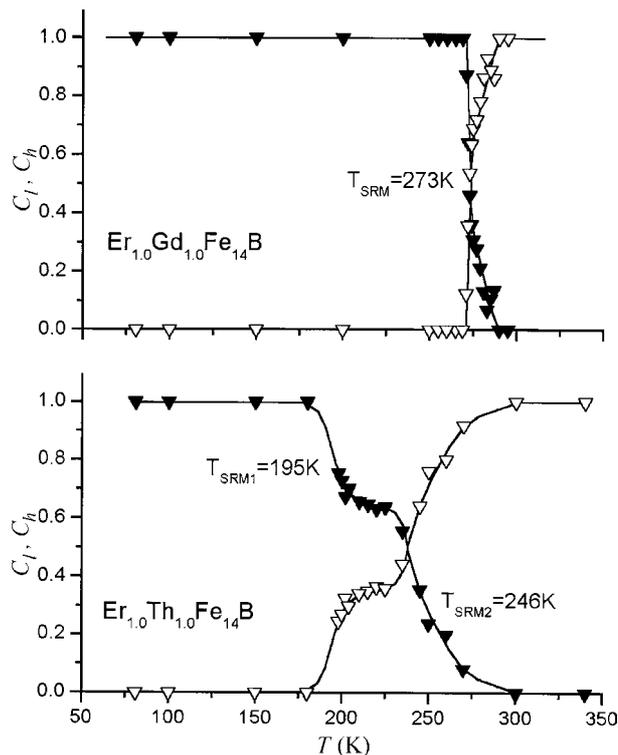
**Fig. 1.** The temperature dependencies of subspectra contributions for  $C_l$  – “low temperature” (solid triangle) and  $C_h$  – “high temperature” (open triangle) Zeeman sextets for  $Er_{1.0}R_{1.0}Fe_{14}B$  (R = Gd, Th).
