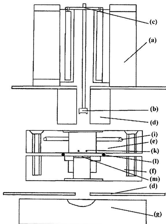
**Fig. 1.** A scheme of the experimental set-up. (a) – Drive in vertical position, (b) – source, (c) – source fixing point, (d) – collimator, (e) – CEMS counter module, (f) – sample holder module, (g) – proportional counter, (i) – gas-in, (k) – anode wires at zero potential, 4 mm from the sample, (l) – o-ring, (m) – sample at high voltage potential ( $\sim -1440$  V).
