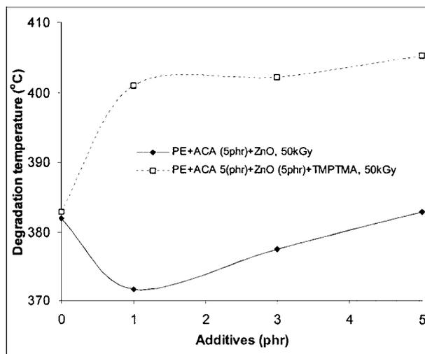
**Fig. 8.** Effect of additives (ZnO, TMPTMA) on degradation temperature of LDPE foam samples, which were cross-linked at 50 kGy.
