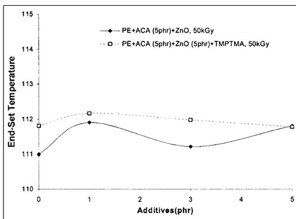
Fig. 6. Effect of additives (ZnO, TMPTMA) on melting end-set temperature of cross-linked LDPE foam samples, which were irradiated at 50 kGy.
