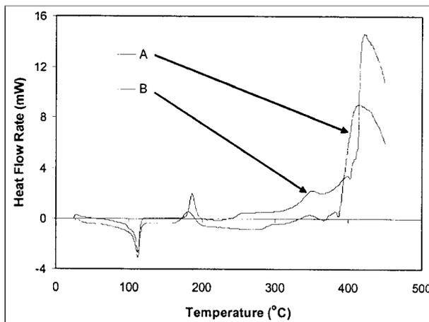
Fig. 4. DSC diagram of LDPE foam samples irradiated at 50 kGy; A – PE + 5 phr of ACA + (1-5) phr of ZnO; B – PE + 5 phr of ACA + 5 phr of ZnO + 1 phr of TMPTMA.
