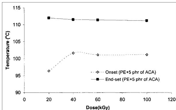
Fig. 2. Effect of radiation dose on melting temperature of LDPE foam samples.
