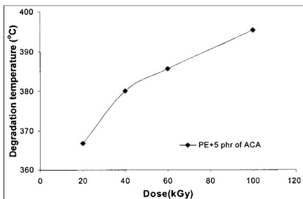
Fig. 3. Relationship between degradation temperature and radiation dose for LDPE foam samples.
