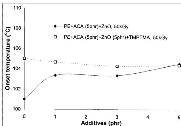
Fig. 5. Effect of additives (ZnO, TMPTMA) on  $T_{mi}$  for cross-linked LDPE foam samples, which were irradiated at 50 kGy.
