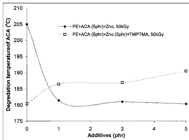
**Fig. 7.** Effect of additives (ZnO, TMPTMA) on ACA degradation temperature in LDPE foams which were irradiated at 50 kGy.
