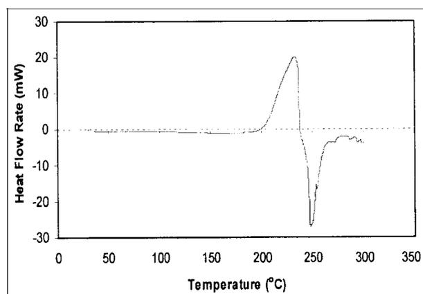
**Fig. 1.** DSC diagram of ACA. Degradation temperature range is 200–220°C.
