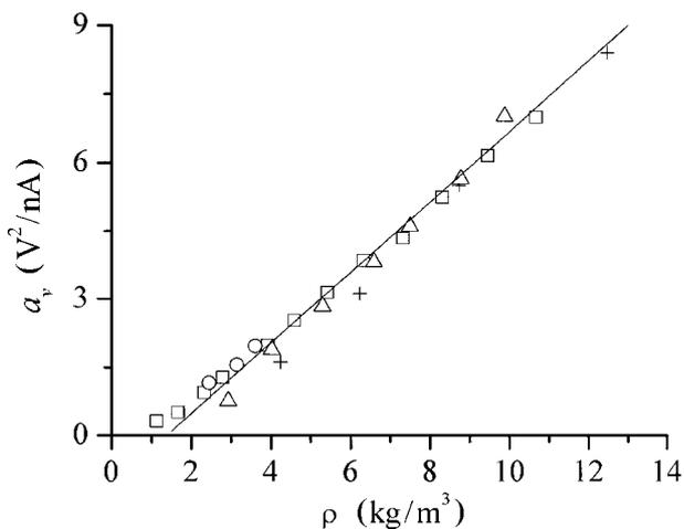
**Fig. 5.** Dependence of the coefficient  $a_v$  on the gas density (squares for methane, crosses for ethane, circles for ethylene and triangles for propane).
