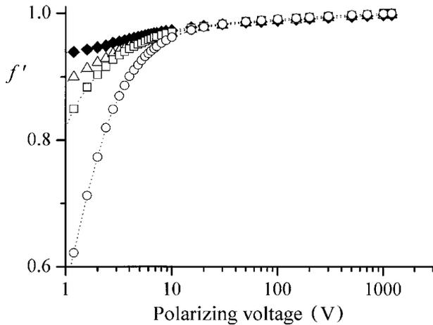
**Fig. 3.** Relative ion collection efficiency measured by the REM-2 chamber filled with methane ( $p = 690$  kPa) and irradiated at two dose rates  $\dot{D}_1 = 5.2$  mGy/h ( $-\circ-$ ) and  $\dot{D}_2 = 0.57$  mGy/h ( $-\square-$ ). Two upper curves represent the results after correction for volume recombination ( $-\triangle-$ ) and also for back diffusion of ions (the upper curve).
