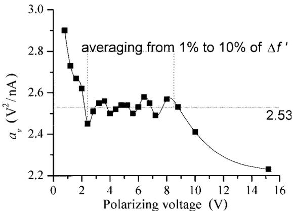
**Fig. 2.** Averaging the coefficient of volume recombination correction  $a_v$  (REM-2 chamber filled with methane,  $p = 690$  kPa).
