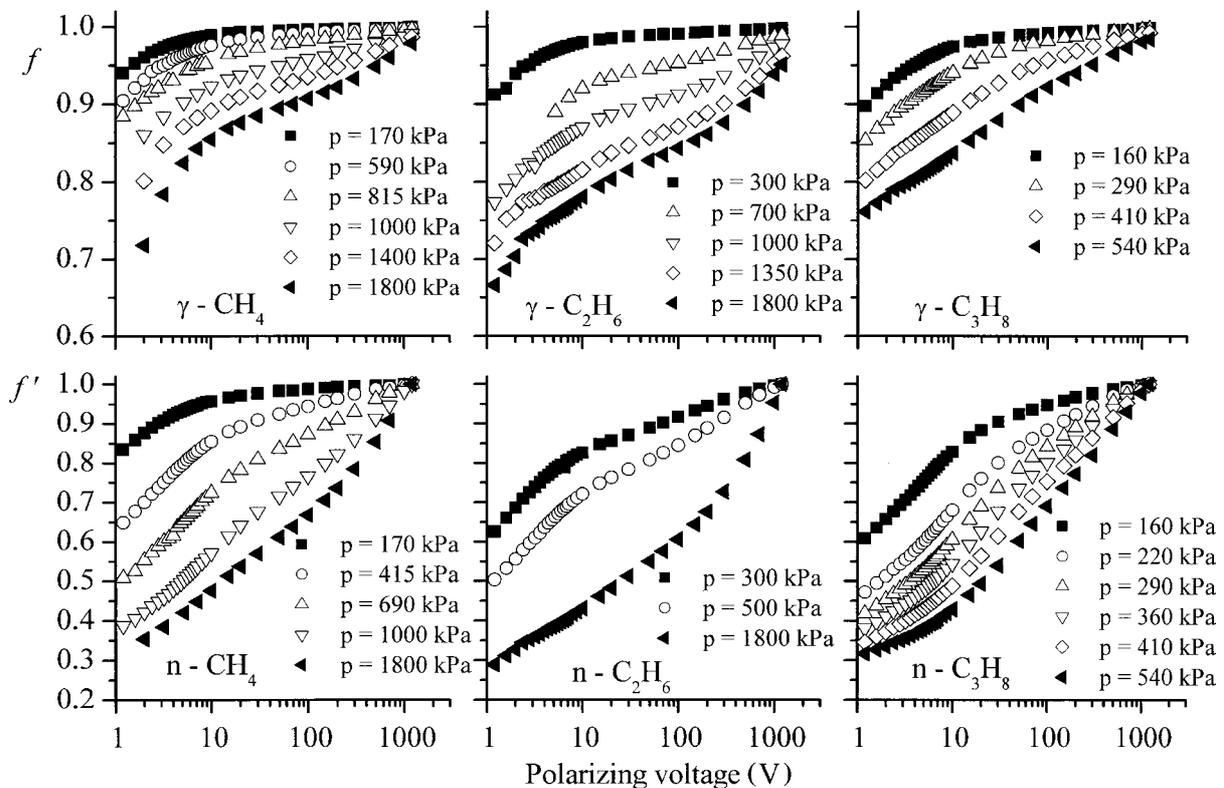
**Fig. 4.** Ion collection efficiency for gamma radiation of <sup>137</sup>Cs source (upper plots) and the relative ion collection efficiency for neutron radiation of <sup>239</sup>Pu-Be source (lower plots) determined by the REM-2 ionization chamber filled with methane, ethane and propane. All curves concern initial recombination, so they do not depend on dose rate.
