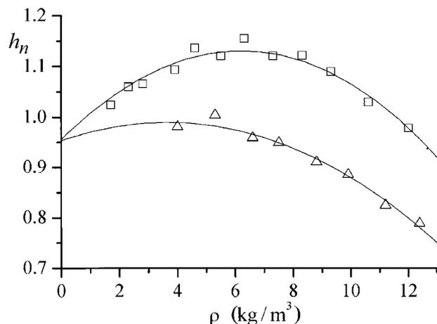
**Fig. 6.** Dependence of relative neutron sensitivity (neutrons from the  $^{238}\text{Pu}$ -Be source) of the REM-2 chamber on filling gas density for methane (the upper curve) and propane (the lower curve).
