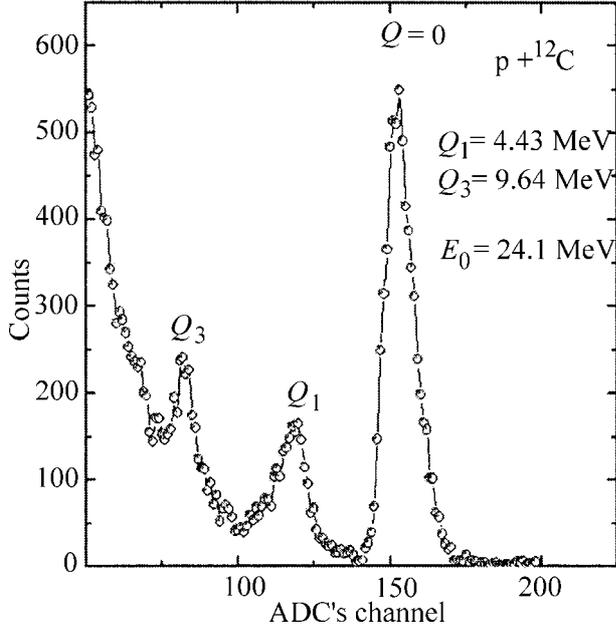
**Fig. 1.** The energy of proton beam  $E_0$  was obtained from the spectrum of protons scattered on  $^{12}\text{C}$  target.
