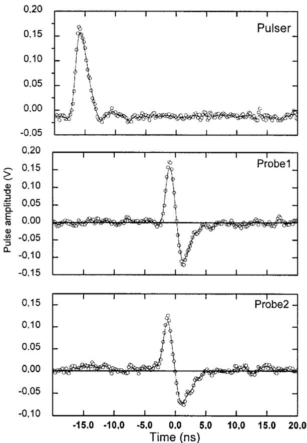
**Fig. 4.** Pulse shapes of generator and corresponding probe pulse.
