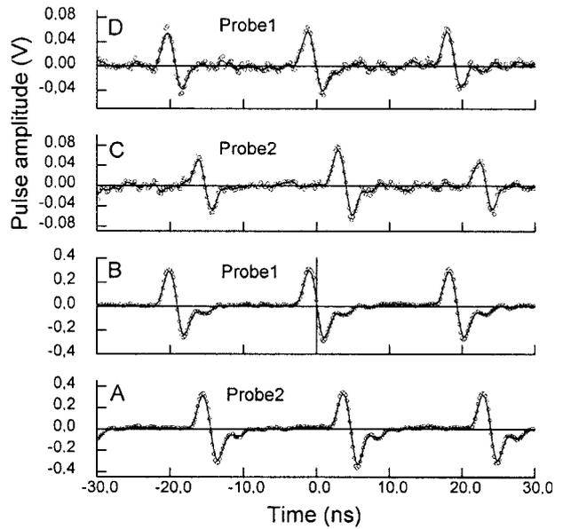
**Fig. 5.** Probes signals induced by 22 MeV proton beam. A-B – beam current 1.5  $\mu$ A; C-D – beam current 0.3  $\mu$ A.
