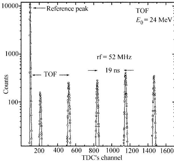
**Fig. 3.** TOF spectrum. The energy of the proton beam  $E_0 = 24$  MeV was obtained from measured velocity.
