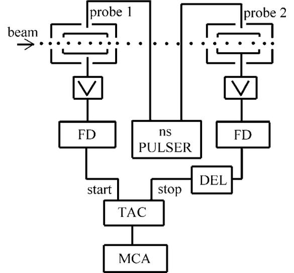
**Fig. 2.** TOF equipment, abbreviations mean: FD – fast discriminator; TAC – time to amplitude converter; DEL – fixed delay in stop channel; MCA – multichannel analyzer.
