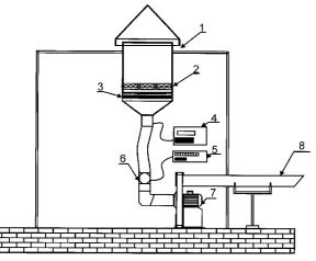
**Fig. 1.** Schematic picture of AZA-1000 set-up. 1 – Suction head cover with air inlet; 2 – 4 infrared heaters; 3 – filter frame tray; 4 – electric box for power supply; 5 – flowmeter display; 6 – flowmeter type VR-600; 7 – air pump high-pressure fan type ZWP-1300 (Venture Industries); 8 – outlet tube.
