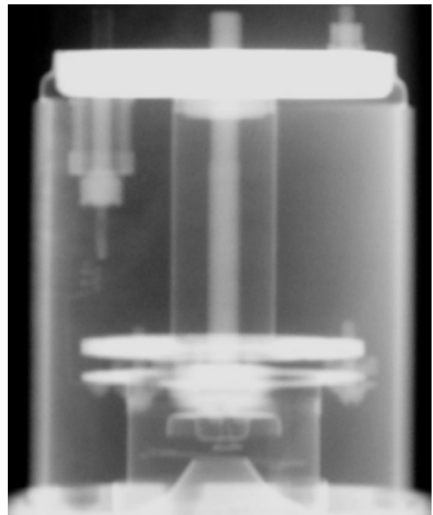
Fig. 9. Radiographic image of the diode electron gun.
