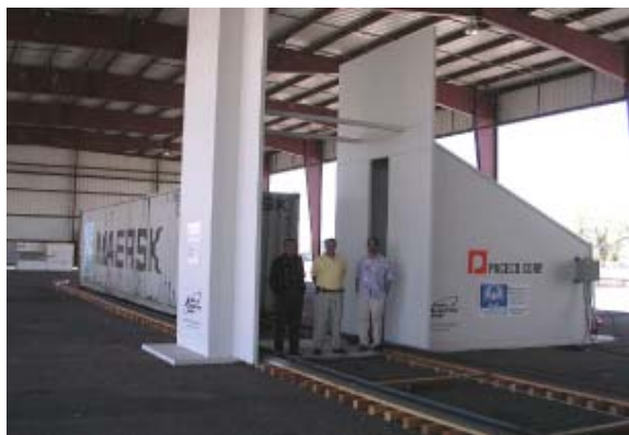
Fig. 7. A prototype of the arrangement of trucks inspection by photofission developed at INEEL in Idaho, USA.
