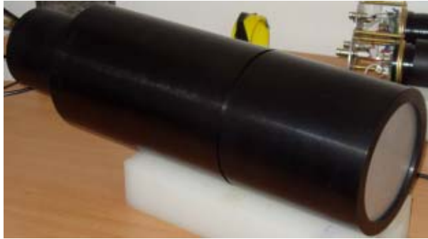
Fig. 10. The developed at IPJ 5" × 5" NaI(Tl) detector done for the EURITRACK system.
