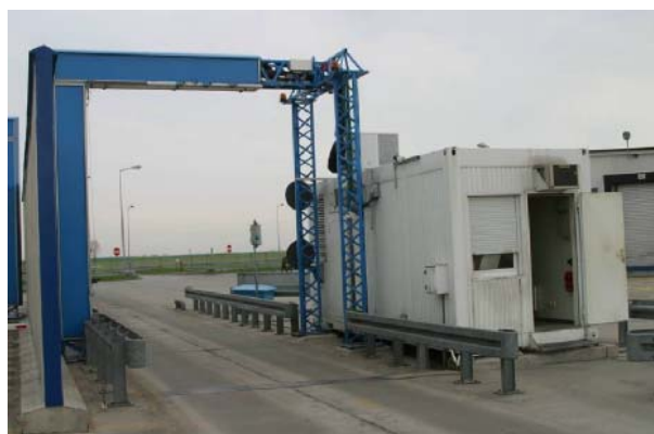
Fig. 8. An X-ray radiography system of trucks monitoring, installed in Terespol, at the Polish-Belarusian border.
