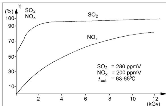
**Fig. 1.**  $\text{SO}_2$  and  $\text{NO}_x$  removal efficiency vs. dose. The results obtained in the pilot plant experiments.
