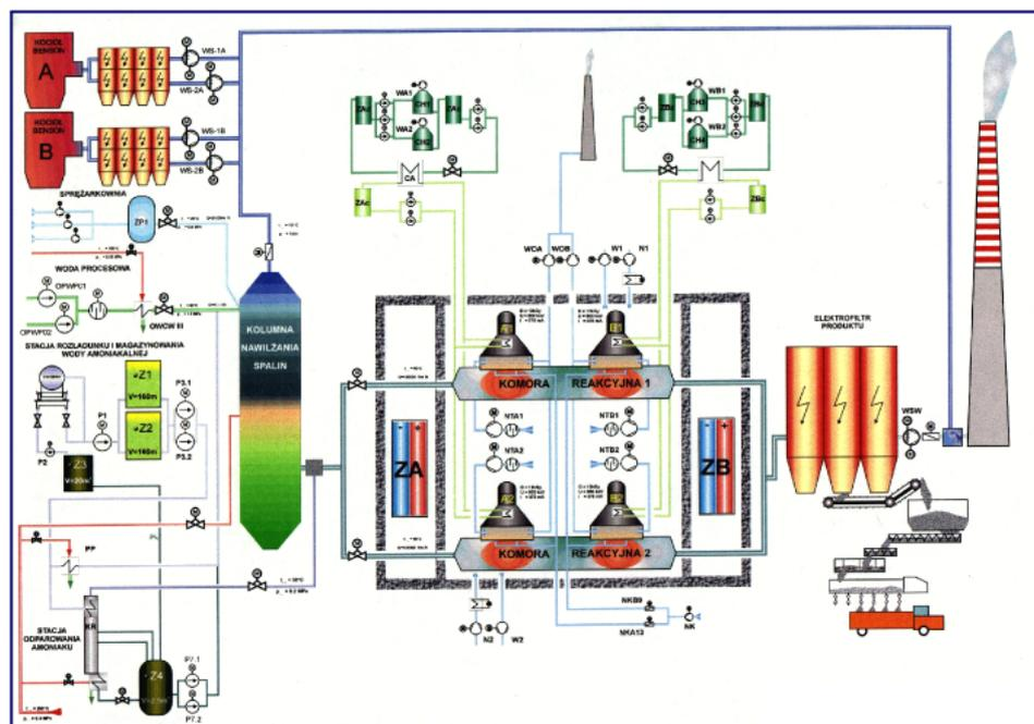
**Fig. 2.** A scheme of the industrial plan for electron beam flue gas treatment at EPS Pomorzany, Poland.
