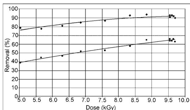
**Fig. 3.**  $\text{SO}_2$  and  $\text{NO}_x$  removal efficiency vs. dose. The results were obtained in an industrial installation. ( $\text{SO}_2$  inlet conc. 1500–1630  $\text{mg}/\text{Nm}^3$ ,  $\text{NO}_x$  inlet conc. 470–540  $\text{mg}/\text{Nm}^3$ .)
