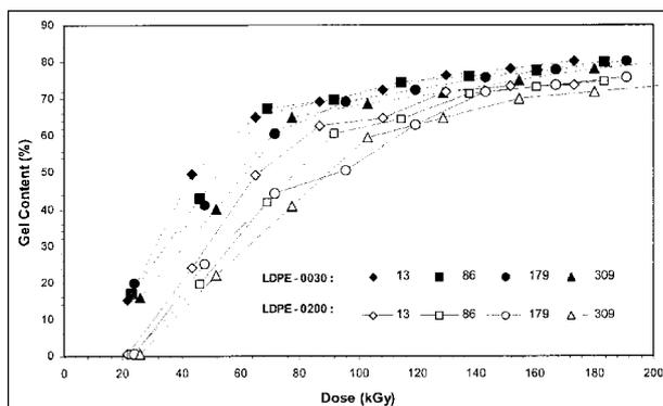
**Fig. 3.** Variations of gel content of the samples as a function of radiation dose. (Dose rate values are also indicated in the legend in kGy/min.)
