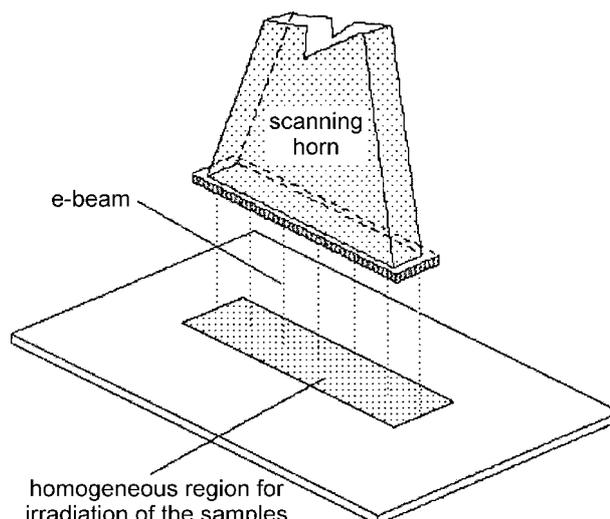
**Fig. 2.** Scheme of the scanning horn and irradiation geometry.
