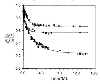
**Fig. 2.** Relative radiotracer quantity *vs.* contacting time for three suspensions differing in CdS and cadmium concentration. The composition of the suspensions (upper, middle and lower lines) in g CdS per 0.24 L and solution concentrations of cadmium in  $\mu$ mol·l<sup>-1</sup> are: 0.30, 132; 0.26, 36; and 2.90, 132; respectively. The lines in the figure are obtained by fitting type (3) equations through the experimental points. The optimal fit was obtained for n = 3.
