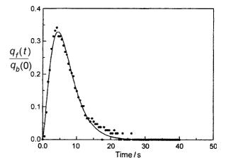
**Fig. 6.** Typical experimental  $q_f(t)/q_b(0)$  values fitted with a three-exponential term function.
