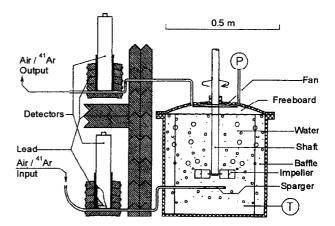
**Fig. 5.** Experimental set-up consisting of a gas-liquid contractor and two lead-shielded radiation detectors.
