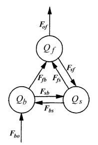
**Fig. 7.** Compartmental model for oxygen transport in a gaswater contactor. Subscripts *o* and *s* denote the outside and solution, respectively.
