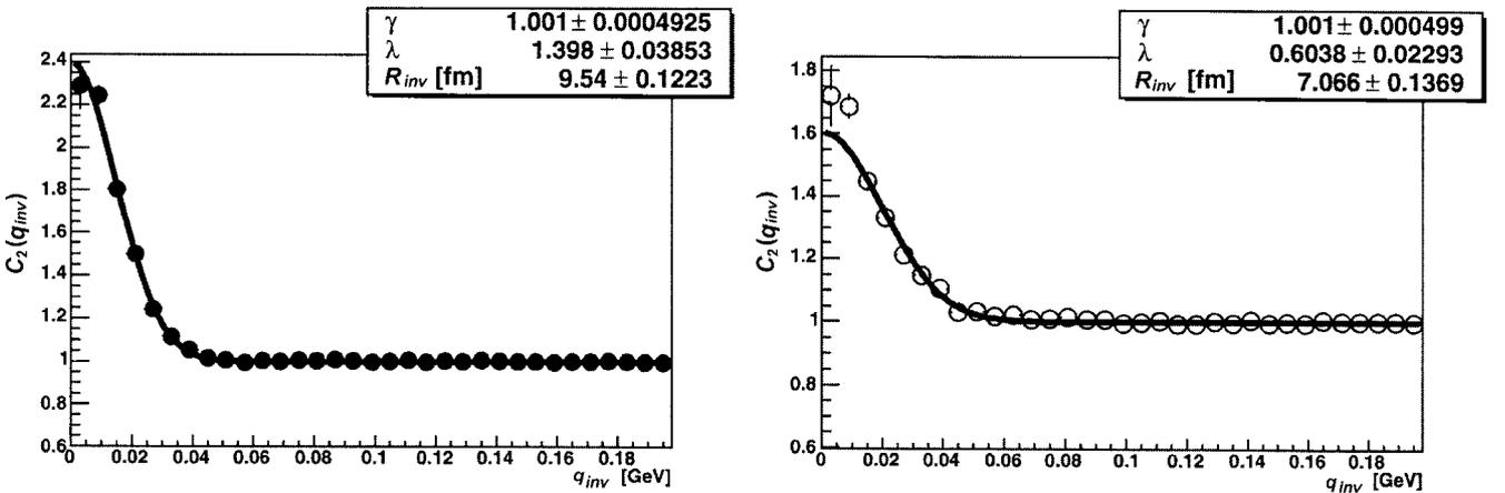
Fig. 1. The  $q_{inv}$  parametrization (2) of the correlation function for  $\pi^+ \pi^-$  pairs using charge reassigning algorithm (left panel) and the weighting method (right panel) with the Gaussian fit.
