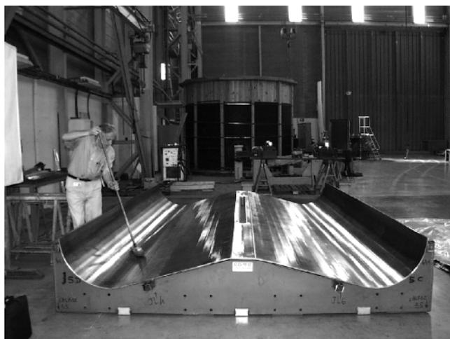
**Fig. 4.** An 8 mm copper sheet placed in the welding jig is cleaned before the electron beam welding of the stainless steel cooling channels.
