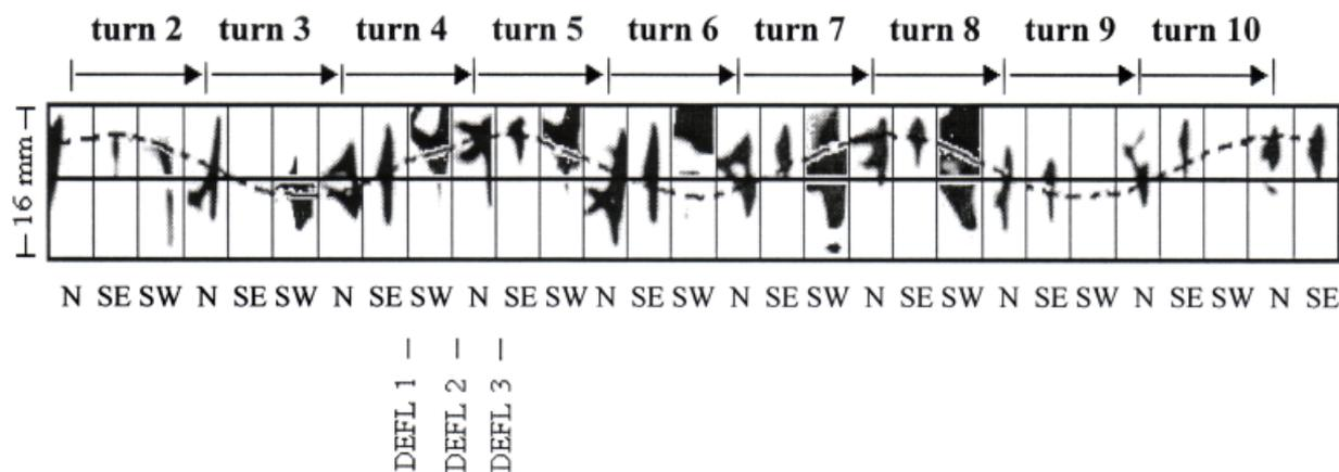
**Fig. 2.** The beam images measured at different occasions on the first turns of JULIC for 45 MeV  $H^-$  ions at extraction. The results indicate a vertical oscillation with an amplitude of close to 4 mm and an unusual pattern of beam-spot shapes. The position of the 3 electrostatic vertical deflectors installed later is also marked.
