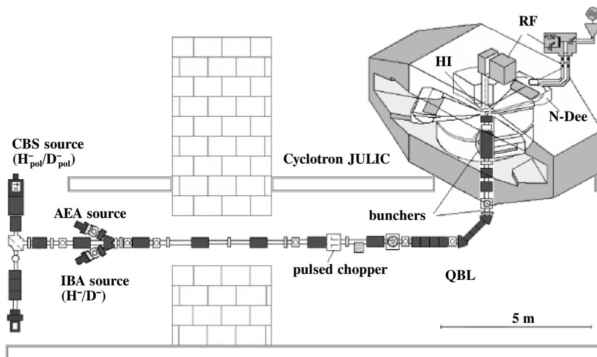
**Fig. 1.** Schematic layout of the cyclotron JULIC as injector of negative ions for the cooler synchrotron COSY, showing the arrangement of the ion sources, source beamline (QBL) and axial injection (compare the text).
