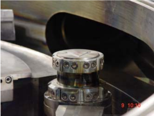
Fig. 3. The beam separator placed in the cyclotron.
