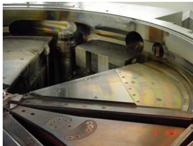
Fig. 2. The extraction path in the cyclotron, with the groove in the long pole, the gradient corrector, the beam separator and the vacuum exit port. The harmonic coils are placed underneath the aluminum outer pole covers.
