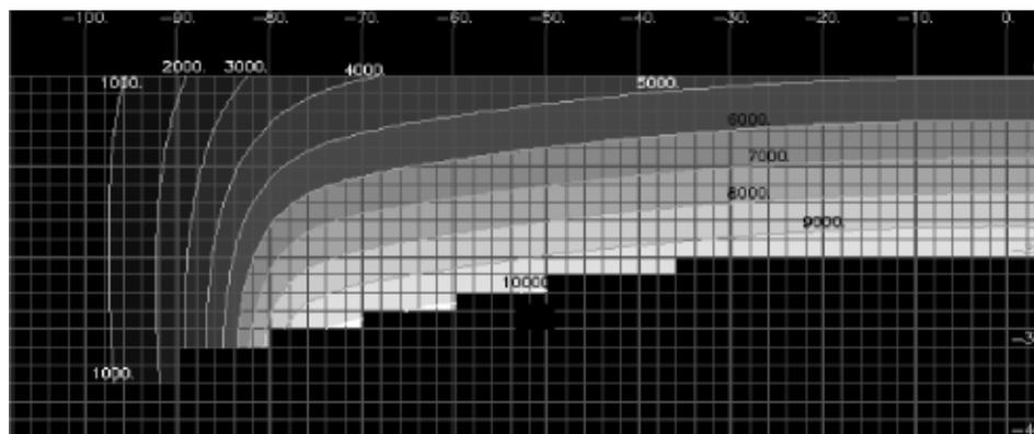
**Fig. 4.** Reconstructed field distribution of the  $B_z$  component in the median plane of the measured on field boundaries  $M_1$  magnet. Reconstruction was based on the experimental data from planes lying at distances  $\pm 30$  mm from the median plane.
