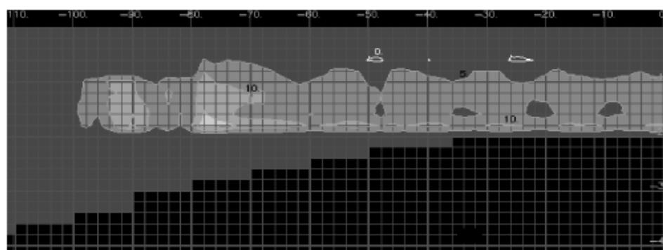
**Fig. 5.** The absolute error distribution of the  $B_z$  ( $\Delta B_z = B_z^{\text{exp}} - B_z^{\text{rec}}$ ) component in the median plane of the  $M_1$  magnet.
