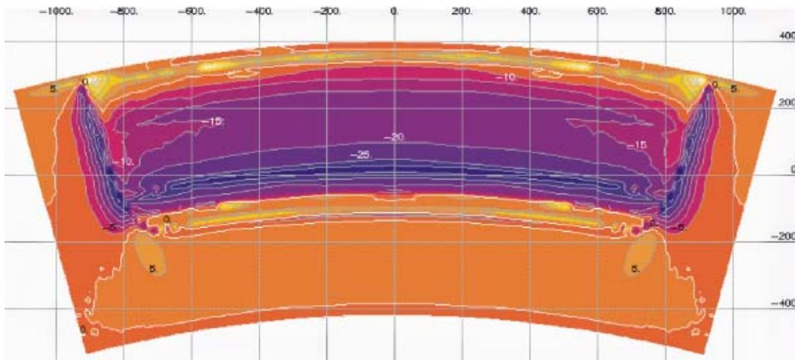
Fig. 7. The absolute error distribution of the  $B_z$  ( $\Delta B = B_z^{\text{exp}} - B_z^{\text{rec}}$ ) component in the median plane of the  $M_2$  magnet.
