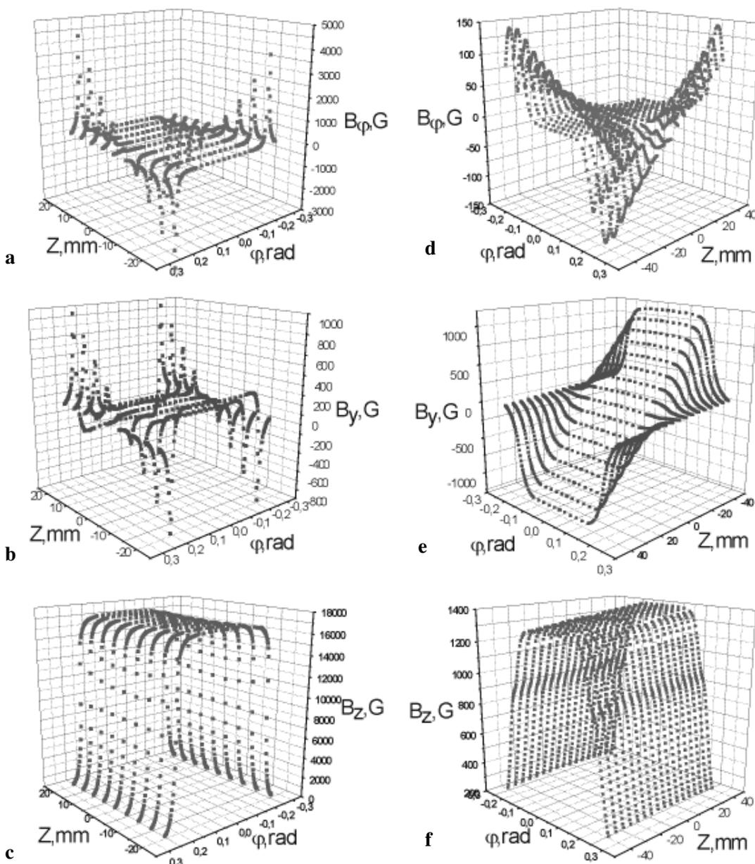
**Fig. 3.** The measured magnetic field distributions of the  $M_2$  magnet at the field value  $B_0 = 11,610$  G. The  $B_\varphi$  (a),  $B_y$  (b), and  $B_z$  (c) are the components of the magnetic field along the border of the maximum radius of the working region and the  $B_\varphi$  (d),  $B_y$  (e), and  $B_z$  (f) are the components of the magnetic field along the border of the minimal radius of the working region.
