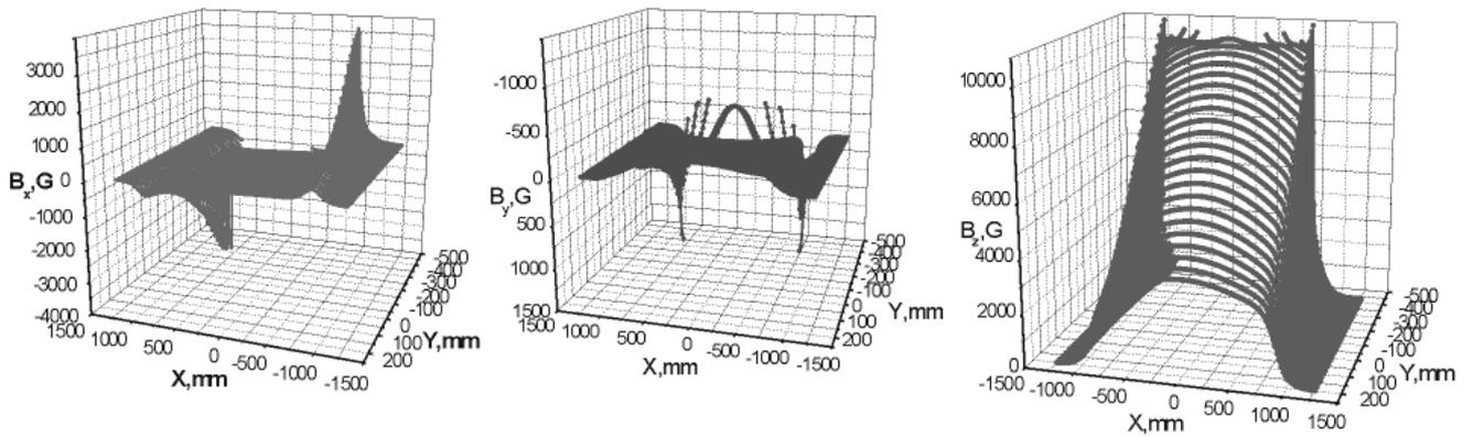
**Fig. 1.** The measured magnetic field distributions of the  $M_1$  magnet at the field value  $B_0 = 7050$  G. The  $B_x$ ,  $B_y$  and  $B_z$  are the components of the magnetic field in the plane lying 30 mm below the median plane.
