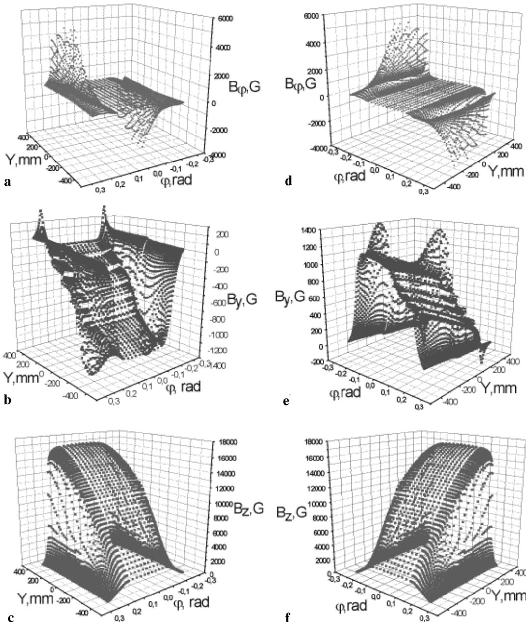
**Fig. 2.** The measured magnetic field distributions of the  $M_2$  magnet at the field level  $B_0 = 11,610$  G. The  $B_\phi$  (a),  $B_y$  (b), and  $B_z$  (c) are the components of the magnetic field close to the upper pole of the magnet and the  $B_\phi$  (d),  $B_y$  (e), and  $B_z$  (f) are the components of the magnetic field close to the lower pole of the magnet.
