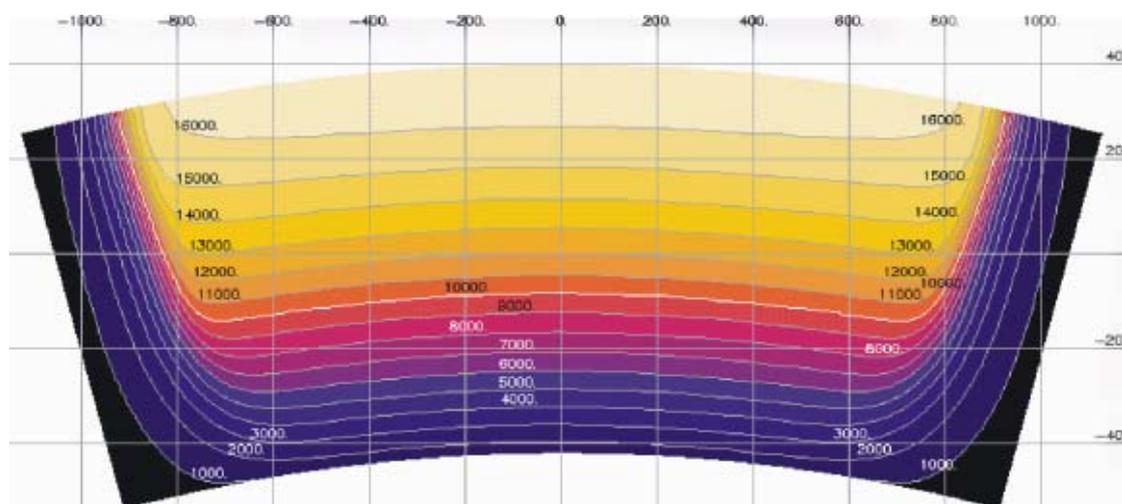
**Fig. 6.** The reconstructed magnetic field distribution in the median plane of the  $M_2$  magnet.
