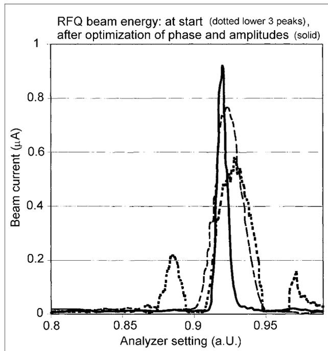
Fig. 3. Analyzing RFQ beam energy.
