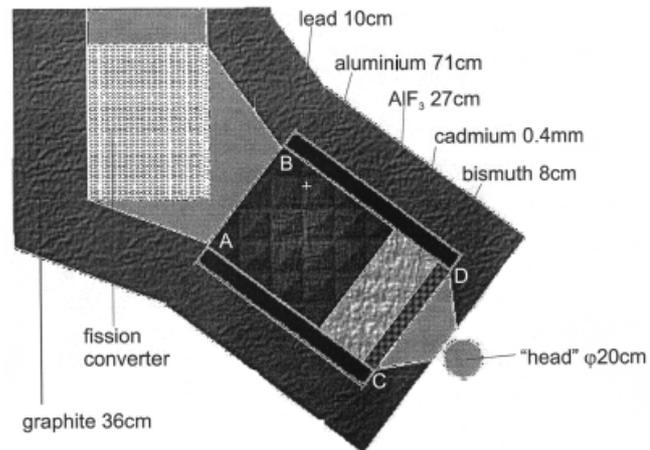
**Fig. 11.** Calculating model of the fission converter (Variant 1A-2) and filter/moderator arrangement (Table 4, Configuration 5).
