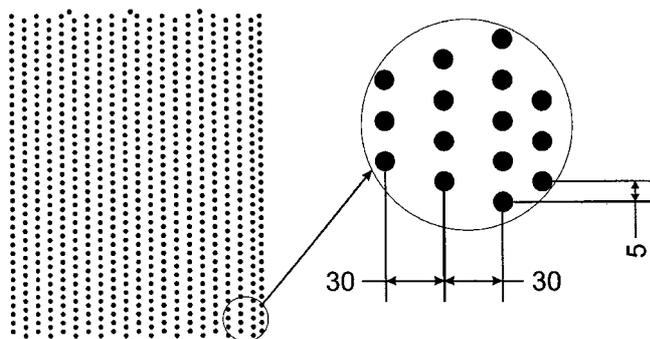
**Fig. 9.** Arrangement of 780 fuel rods EK-10 for Variant IA-2. The rods are placed in 37 rows – 10 and 11 rods alternately, the last row contains only three uranium rods.
