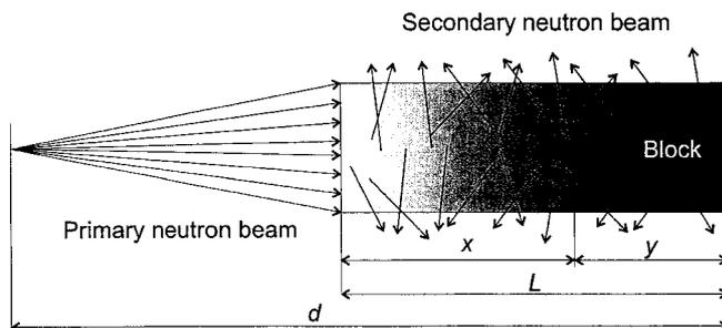
**Fig. 1.** A scheme of the analysis for the homogenisation of the neutron flux.
