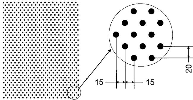
**Fig. 8.** Arrangement of 780 fuel rods EK-10 for Variant IA-1. Each rod contains 8.045 g of  $^{235}\text{U}$  the rods being arranged in 39 rows with 20 rods in every row, which correspond to 6275 g of  $^{235}\text{U}$ .
