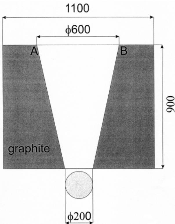
Fig. 5. A graphite shield of the filter.
