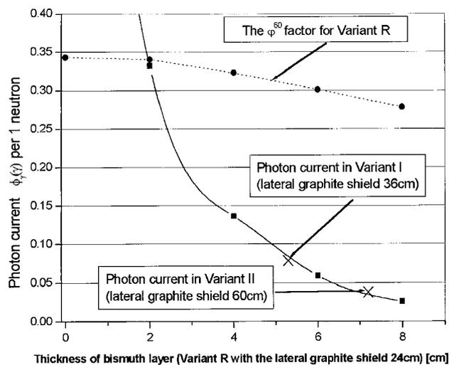
Fig. 6. Photon current in a function of the thickness of bismuth layer in Variant R. Variants I and II are comparable to Variant R with 6 cm of bismuth. Dashed line:  $\phi^{60}$  factor for Variant R.
