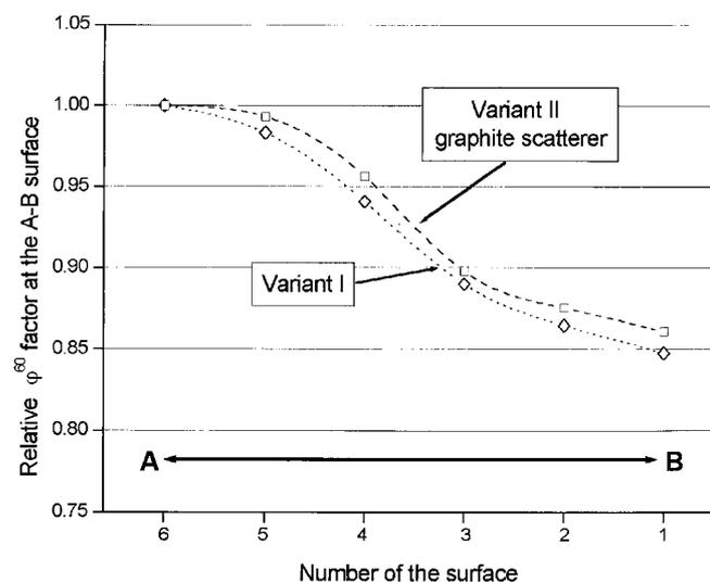
Fig. 7. Distribution of the relative  $\phi^{60}$  factor along the A–B surface for Variant I and II.
