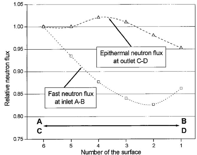
**Fig. 10.** Distribution of the relative fast and thermal neutron fluxes at the inlet A–B and the outlet C–D of the filter/moderator system. Variant IA-2 of the converter, Configuration 4j of the neutron filter/moderator.
