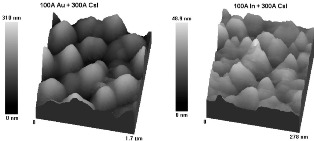
**Fig. 3.** Difference between the surfaces of the  $\text{Si}_3\text{N}_4$  membrane covered with the CsI layer evaporated on In (right) and on Au (left) conductive layer. Please note the significant difference in scale.
