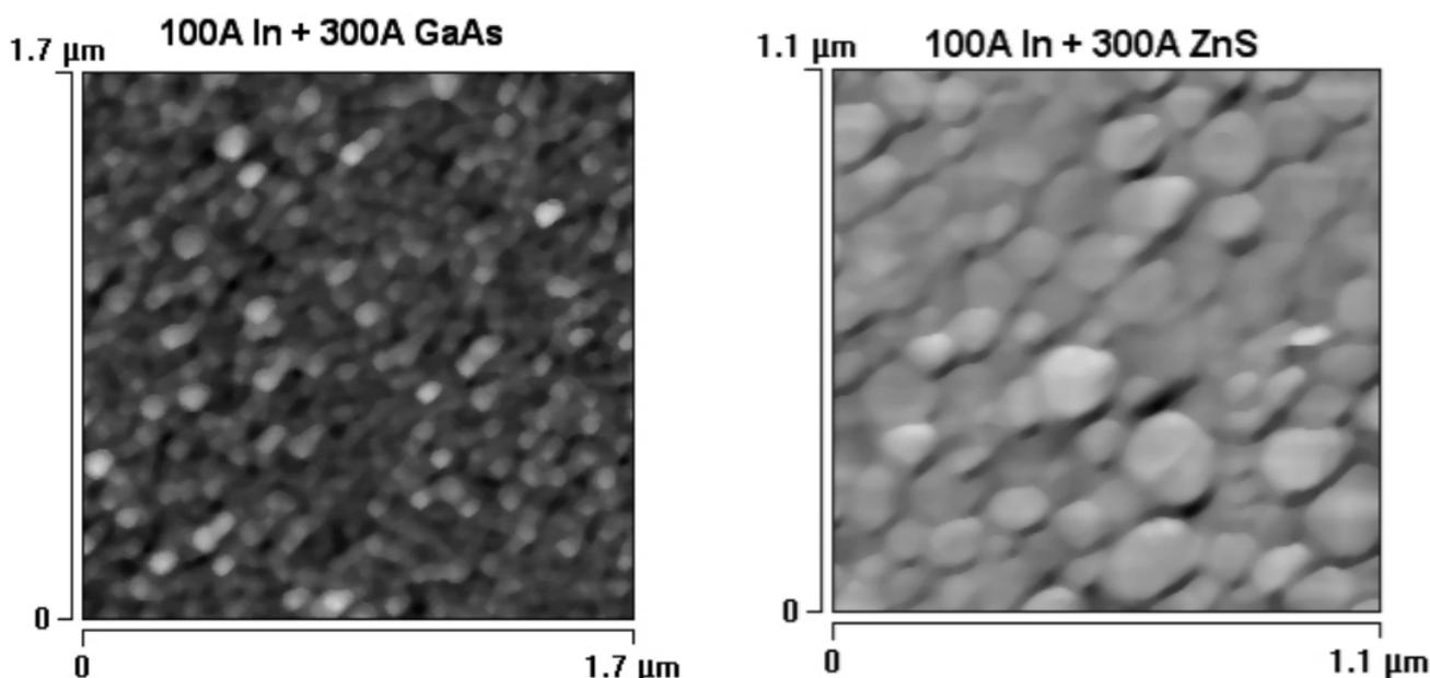
**Fig. 2.** SFM images of a Si<sub>3</sub>N<sub>4</sub> membrane surface covered with GaAs (left) and ZnS (right). Please note the different scanning areas.
