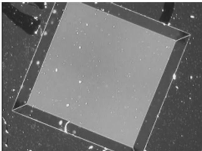
**Fig. 1.** Microscope image of the window with the Si<sub>3</sub>N<sub>4</sub> membrane covered with a gold layer.
