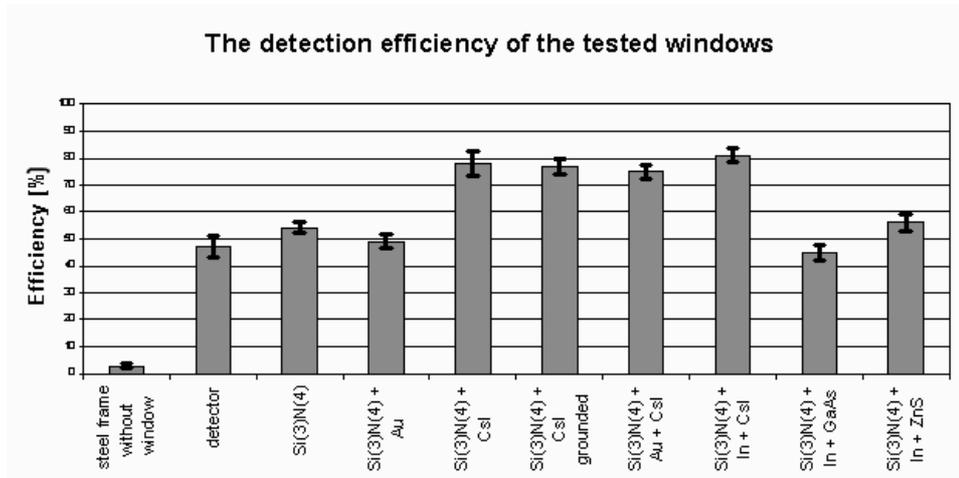
**Fig. 7.** The chart of the membranes efficiency for the alpha particles registration – all  $\text{Si}_3\text{N}_4$  membranes were 200 nm thick. The Au and In conducting layers were 10 nm thick. The CsI, ZnS, GaAs layers were 30 nm thick. In most cases two different windows of the same covering were investigated.
