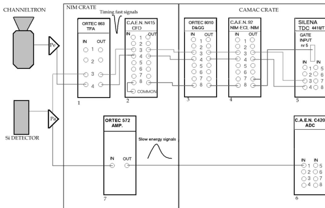
**Fig. 5.** Data acquisition system. Pe – preamplifier for channeltron signals. Pa – preamplifier for timing and energy signals from Si detector (ORTEC 2398). 1 – timing filter amplifier; 2 – constant fraction discriminator; 3 – delay and gate generator; 4 – NIM-ECL-NIM translator; 5 – time to digital converter; 6 – amplitude to digital converter; 7 – active filter amplifier.
