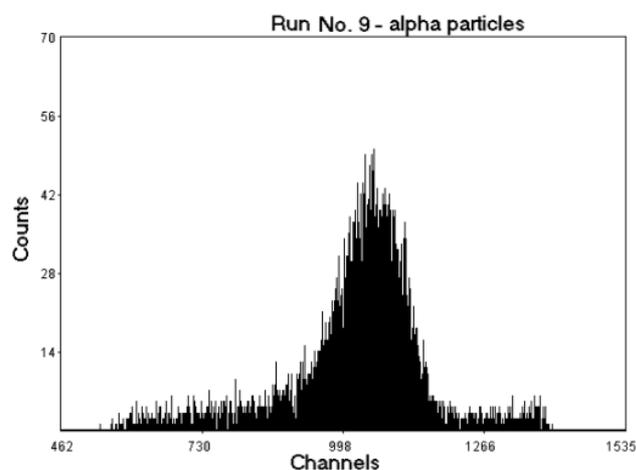
**Fig. 6a.** Energy spectrum of  $^{241}\text{Am}$  alpha particles detected after the passage through membrane. Channel width is 5.37 keV.
