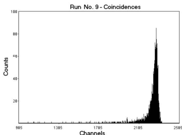
**Fig. 6b.** Time spectrum (coincidences between alpha particles and electrons). Channel width is 250 ps.
