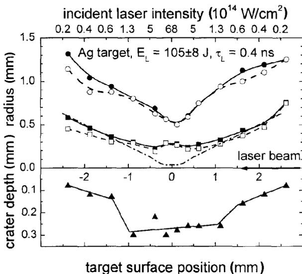
Fig. 4. The radii of craters (■, □ – maximum and minimum radius of crater), damages (●, ○ – maximum and minimum radius of damages), depth of crater (▲ – depth of craters) and the caustic of focusing lens (--- – caustic of the focusing lens) as a function of the target surface position.
