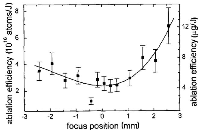
Fig. 5. The ablation efficiency of silver.
