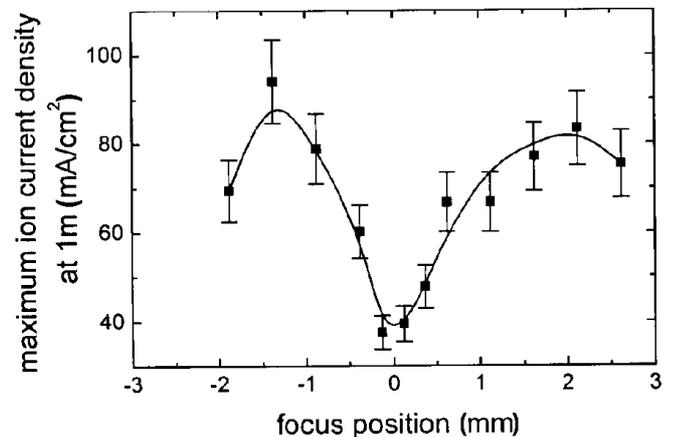
Fig. 3. The maximum ion current density at the distance of 1 m from the target.
