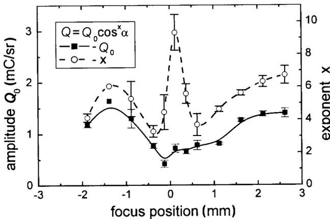
Fig. 1. The amplitude  $Q_0$  and exponent  $x$  of the angular distribution of silver ions.
