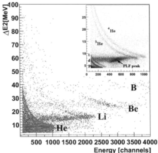
Fig. 2. Identification matrix for  $^{17}\text{O}+^{131}\text{Xe}$  reaction at 250 MeV/nucleon taken with Si-Si-CsI telescope at  $6.8^\circ$ . Insert shows  $^3,^4\text{He}$  resolution and  $Z=1$  region.
