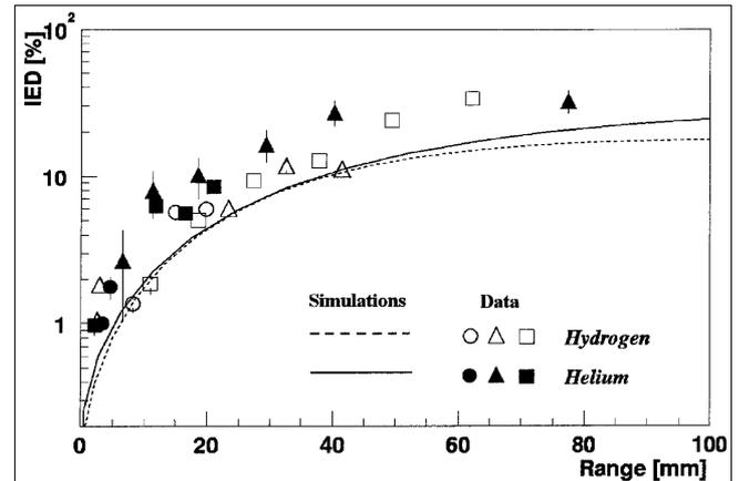
Fig. 7. The percentage contribution of IED events as a function of particle range in CsI(Tl) scintillator. Points and lines have the same meaning as in Fig. 6.
