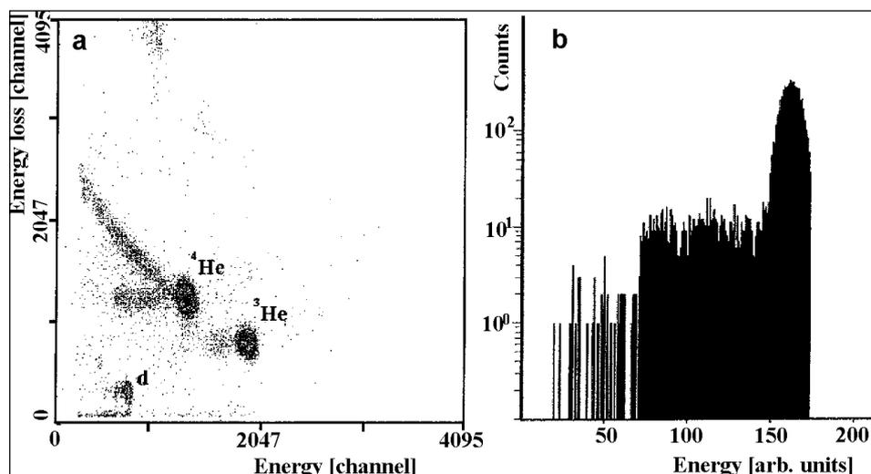
Fig. 1. Identification matrix from measurements on ACCULINNA separator (left-hand side). Energy spectrum of alpha particles at 94 MeV (right-hand side).
