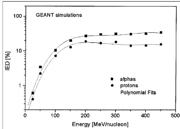
Fig. 5. Energy dependence of the percentage contribution of IED events for protons (circles) and alpha particles (squares) simulated with GEANT (points) and fitted with 4<sup>th</sup> order polynomial (solid line).
