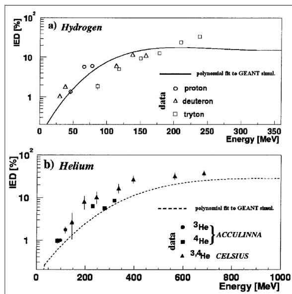
Fig. 6. Comparison of experimental data with MC simulations for hydrogen – a), and helium – b) as a function of their initial energy. Points represent experimental data, lines are polynomial fits to GEANT simulation.
