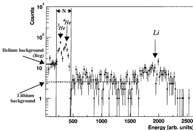
Fig. 3. Experimentally obtained energy spectrum for  $16\text{ MeV} < \Delta E2 < 18\text{ MeV}$  with marked helium and lithium backgrounds.
