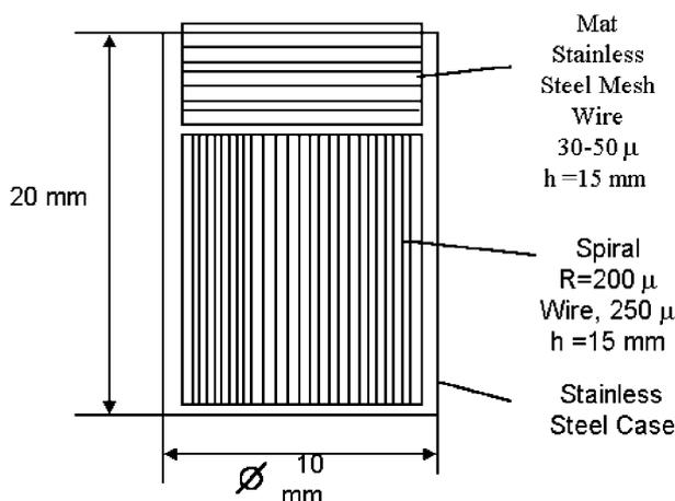
Fig. 3. Scheme of CPS sample.
