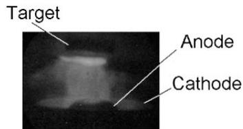
Fig. 6. The formation of a plasma layer near the sample surface.
