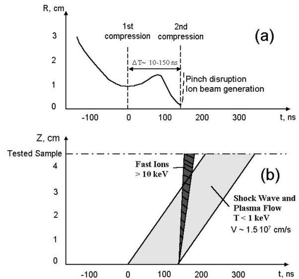
Fig. 7. The sequence of the processes in PF: (a) – R-t diagram of the pinch dynamics, R – radius of pinch, (b) – dynamics of the ion beam and the axial plasma flows.
