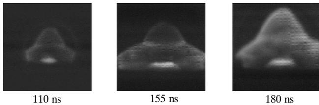
Fig. 5. Pinhole images of PF in visible light, as registered with the 3 ns exposition. “Zero” time instant corresponds to the maximum of the pinch compression (the first compression).
