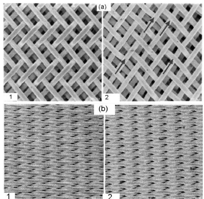
Fig. 4. Two types of the CPS samples (a and b): 1 – before the test, 2 – after the test. Arrows show some disturbances which arose during the tests.
