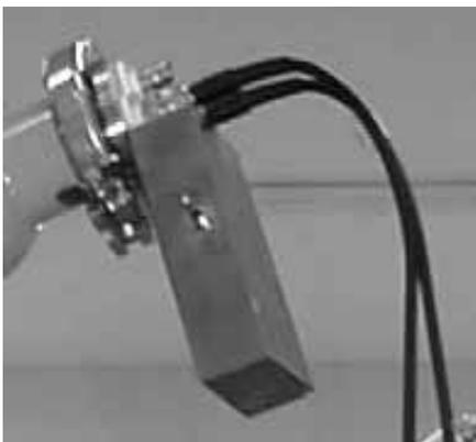
Fig. 4. View of the detection head mounted at the experimental chamber. The attached cuboidal box contains DC/DC converter and battery.
