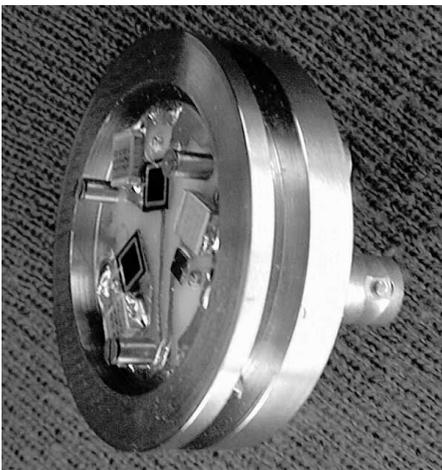
Fig. 3. Side view of the detection head (without DC/DC converter and after removing the plate that supports filters).
