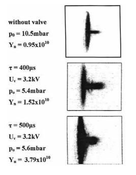
Fig. 3. Soft X-ray pinhole pictures, which were taken with a pinhole camera from discharges performed in the PF-360 facility with the gas puffing, at  $U_0 = 30 \text{ kV}$  and  $W_0 = 122 \text{ kJ}$ . The figure makes possible to perform a comparison of pictures taken for shots without and with  $D_2$  puffing at different values of a time delay ( $\tau$ ).
