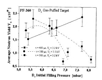
Fig. 2. Average neutron yields versus the initial deuterium pressure, as measured for PF-360 experiments performed with additional gaspuffed targets at  $U_0 = 30 \text{ kV}$  and  $W_0 = 122 \text{ kJ}$ . The different values of valve time shift ( $\tau$ ) and valve voltage ( $U_v$ ) were applied.
