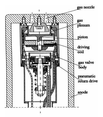
Fig. 1. Assembly of a fast high-pressure gas valve, as designed for gas puffing experiments with the PF-360 facility.
