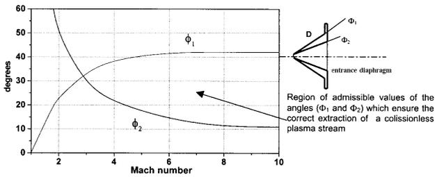
Fig. 3. Dependence of the outer angle ( $\Theta_1$ ) on the inner angle ( $\Theta_2$ ) of the input conical diaphragm on the Mach number ( $M$ ) of the analyzed plasma stream [7, 9].
