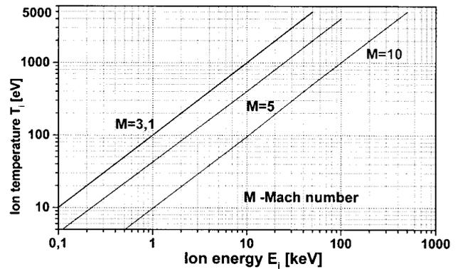
Fig. 4. Relation between the ion temperature ( $T_i$ ) and a parallel component of the ion energy ( $E_{i||}$ ), as determined for plasma streams with different Mach number [14].
