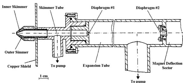
Fig. 6. Scheme of an ion extractor system used for studies of ion beams generated by a plasma-focus machine [5].
