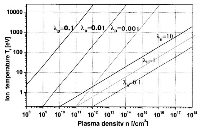
Fig. 2. Relation of the ion temperature ( $T_i$ ) and the plasma concentration ( $n$ ) for different values of the Debye radius ( $\lambda_D$ ) and the ion free path ( $\lambda_{ii}$ ).
