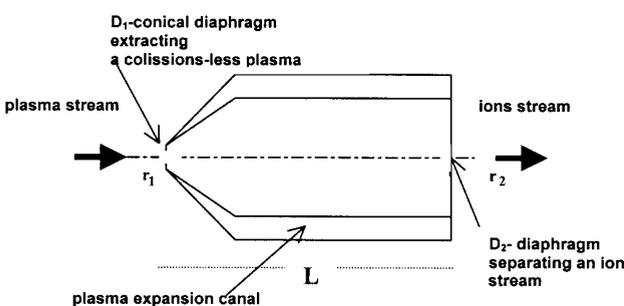
Fig. 1. Scheme of an input diaphragm system used for the extraction of ions from a dense plasma stream.
