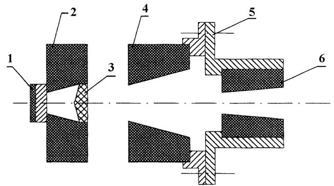
Fig. 1. Schematic diagram of whole the collimator system. 1 – target, 2 – primary collimator, 3 – flattening filter, 4 – secondary collimator, 5 – narrow beam collimator holder, 6 – narrow beam collimator.
