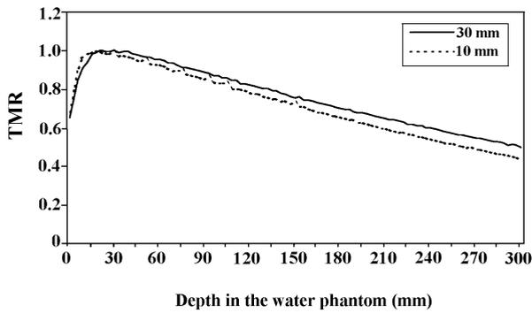
Fig. 2. Tissue maximum ratio (TMR) of 15 MV photon beam, measured for 10 and 30 mm collimator diameters with the 0.12 cm<sup>3</sup> ion chamber.
