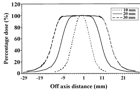
Fig. 3. Beam profiles (OAR) of 15 MV photon beam formed with collimators of 10, 20 and 30 mm in diameter, measured with the 0.12 cm<sup>3</sup> ion chamber.
