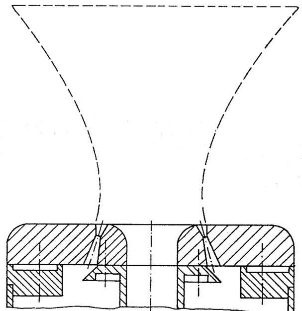
Fig. 2. Cross-section of the inner electrode (anode, 131 mm diameter) with nozzles (diameter 2 mm, tilted by 15° to the axis). The pinch region is marked by the dotted lines.
