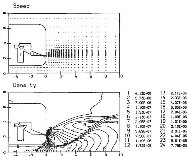
Fig. 3. Plots of distributions of flowing speed and gas density at 400 μs after the opening of the valve. Radial and axial scales are given in cm.
