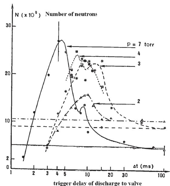
Fig. 6. Neutron yields for shots with various equilibrium chamber filling pressures (reached after about 100 ms) from 2 to 7 Torr deuterium, accomplished with gas puffing in the breakdown region. The valve opened 4 times for 1 ms about every 10 ms. Plotted results are averaged over 10 shots [1]. Neutron yield with static filling amounts to  $10^9$  for  $p = 3$  Torr, as indicated by the broken horizontal line.
