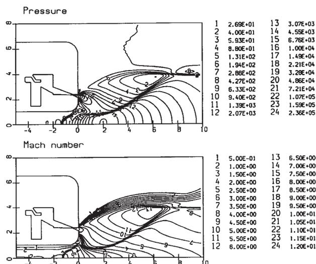
Fig. 4. Contour plots as in Fig. 3 for gas pressure and Mach number, also at 400 μs after the opening of the valve.
