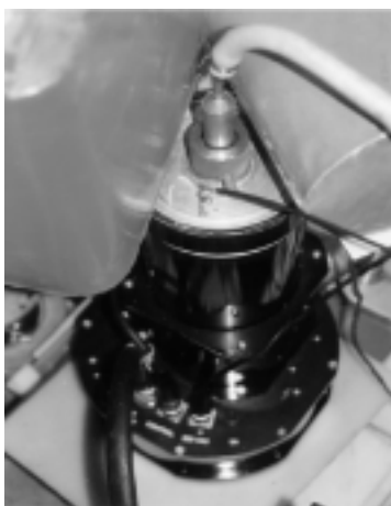
Fig. 3. DPF chamber intended to generate hard X-ray radiation (on the left) and the opened DPF chamber.
