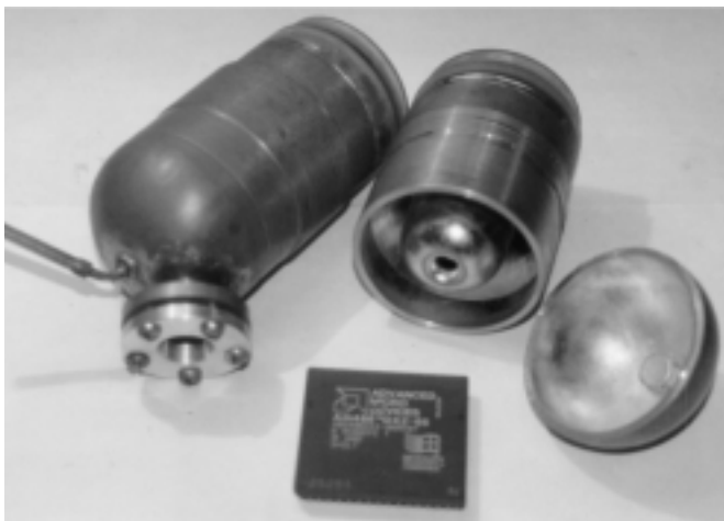
Fig. 3. DPF chamber intended to generate hard X-ray radiation (on the left) and the opened DPF chamber.
