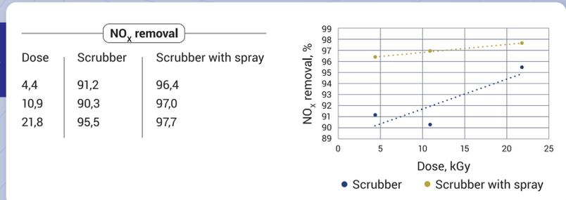
Figure 2. Comparison of NO<sub>x</sub> removal efficiency for scrubber with water spraying to the reactor and sole scrubber
