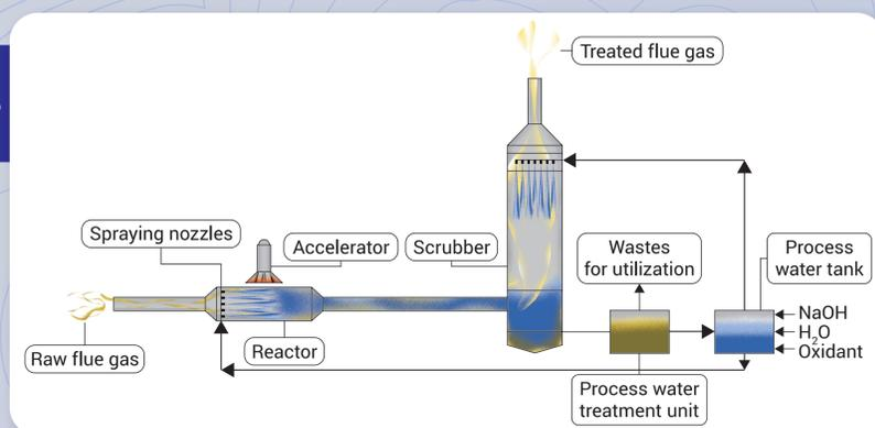
Figure 1. Flue gas treatment installation scheme according to the invention
